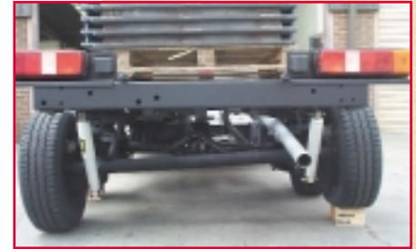
TAG axle weighted with 1750kg of steel plate. Load remains level with 100mm of travel
