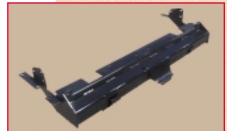
The 6x2 dedicated, heavy duty – 2300 kg tow hitch (optional extra) features 18 mounting points, flat & square tongues, plus both 7 pin & round sockets on each tow bar.
