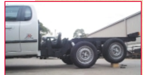
Maximum traction at all times. Shown with 100mm block placed under rear axle.
