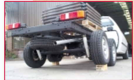
The new 6x2 TAG axle has greater diagonal flexibility. This means less strain on the chassis & improved driver comfort.
